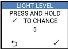
Press and hold the RIGHT button ("✓") to adjust the brightness of the LED light ring; the screen text will flash 3 times to indicate that the setting is ready to be adjusted.
