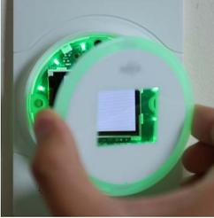
In the event Setra Lite needs to be removed for service, first remove the front lens. To remove the front lens, grab the front lens from the left and right side edges, and pull the lens away from the wall.
