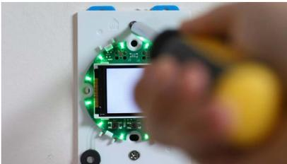
4. Push Setra Lite into the enclosure and secure with two (2) mounting screws.
