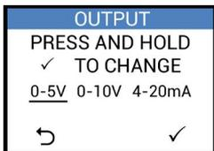
Press and hold the RIGHT button ("✓") to change the output type. The screen text will flash 3 times to indicate that the setting is ready to be adjusted.
