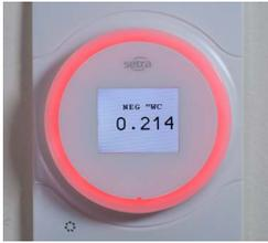
To silence audible alarm, press the light ring below the display. Audible alarm will stop but red status light will maintain until pressure is within set limits one time
