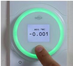
If the DISPLAY is set to "OFF", the LCD display will display Setra logo under normal operation. To see a digital pressure reading, simply press on the lens of Setra Lite.
