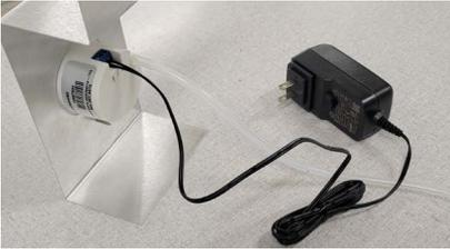
4. Connect pressure tubing from the Pressure Pickup Port to the port on the back of Setra Lite.
