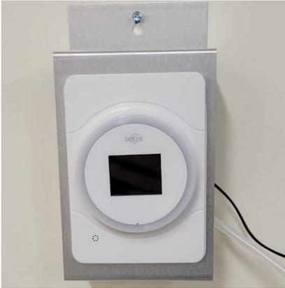
9. If mounting to wall install a screw in the wall via drywall anchor or screwing into a supportive structure leaving the screw protruding approximately 1/8" (3mm). Place quickmount onto screw, then tighten screw until firmly tightened.
