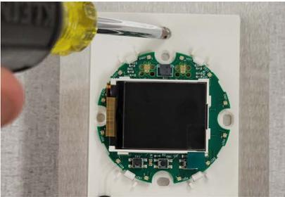
6. Install the Setra Lite base unit housing into the metal quick mount bracket with the provided machine screws.
