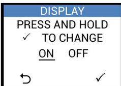
Press and hold the RIGHT button ("✓") to adjust display behavior (i.e. whether the LCD display shows the digital pressure reading by default); the screen text will flash 3 times to indicate that the setting is ready to be adjusted.
