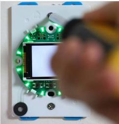
Once the faceplate has been removed, unscrew the unit from the wall or electrical box, and disconnect wires and pressure tubing.
