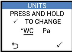
Press and hold the RIGHT button ("✓") to adjust the measuring units used for the digital display and alarm thresholds; the screen text will flash 3 times to indicate that the setting is ready to be adjusted.
