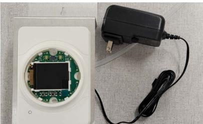
8. Install the faceplate by firmly pressing it into place over the base unit housing.
