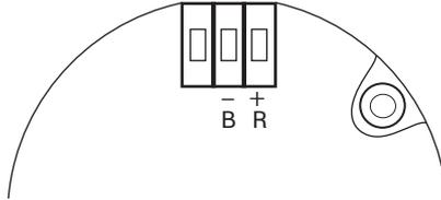
The power connection for Setra Lite uses the 2 pins on the right when looking at the rear of the unit. Connect the 24 VDC (+/- 10%) or 24 VAC (18-32 VDC operational), 50-60 Hz lines to the terminals marked above typically black (B) and red (R) wire.
