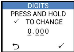
Press and hold the RIGHT button ("✓") to adjust the number of decimal places displayed on the LCD screen; the screen text will flash 3 times to indicate that the setting is ready to be adjusted.
