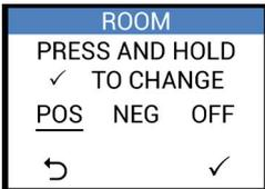
Press and hold the RIGHT button ("✓") to adjust the room (i.e. whether the room is positively or negatively); the screen text will flash 3 times to indicate that the setting is ready to be adjusted.
