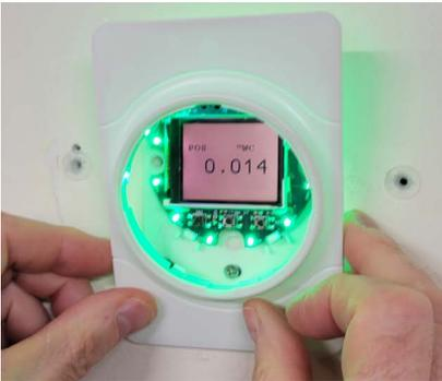
7. Install the faceplate by firmly pressing it into place over the base unit housing.
