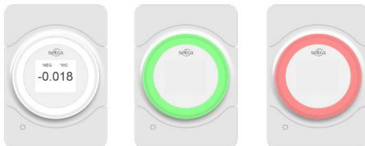
Setra Lite features an LED light ring that will glow red and/or audibly alarm if room pressurization exceeds the configured alarm threshold. With a simple press of the front lens of the unit, the LCD displays the current differential pressure and silences the audible alarm. Configuration of the unit can be performed on the device via buttons located behind the removable front lens. The unit can be put into and taken out of "Standby" mode by pressing the front lens 3 times in quick succession.
