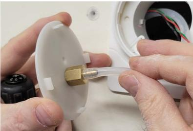
5. Push the open end of the supplied tubing onto the port on the back of the dual alert pressure pickup.
