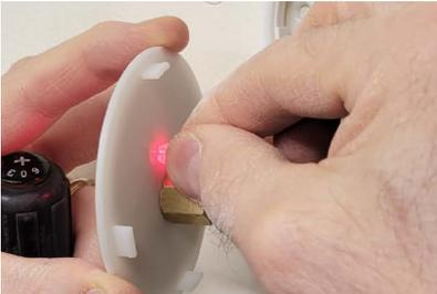
6. Press the LED wire lead into the open hole in the center of the dual alert pressure pickup until it firmly seats into the back of the plate.
