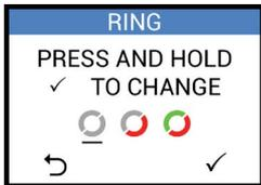
Press and hold the RIGHT button ("✓") to select between no ring light, alarm (red) ring light only or both green/red light ring indicators. The screen text will flash 3 times to indicate that the setting is ready to be adjusted.
