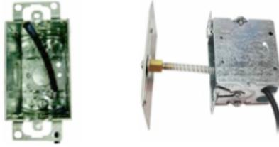
1. Install the supplied silicone tube (with integrated external spring) and attached barbed tube adapter on the rear face of the RPS unit onto the end of the 0.25" field tubing. This short length of tubing is used as a safety to prevent any kinking inside tight spaces. Add your typical run of 1/8"ID x 1/4"OD tubing between the pressure pickup and the Setra Lite.
