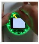
Next, locate the 4 snaps holding the faceplate to the unit. Carefully push on the inside lip of the faceplate near each snap to disengage each snap one at a time.
