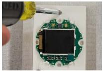
Install the Setra Lite base unit housing into the metal quick mount bracket with the provided machine screws.
