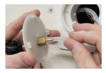
5. Push the open end of the supplied tubing onto the port on the back of the dual alert pressure pickup.
