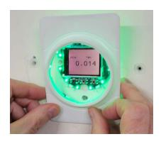
7. Install the faceplate by firmly pressing it into place over the base unit housing.
