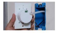
Connect pressure tubing from the Pressure Pickup Port to the port on the back of Setra Lite.
