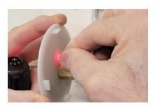
Press the LED wire lead into the open hole in the center of the dual alert pressure pickup until it firmly seats into the back of the plate.
