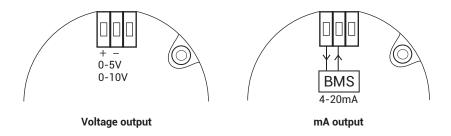
If using the Analog Output (AO) for voltage output, connect to the terminals as labeled on the left diagram above. If using the AO for mA output, connect to the terminals shown in the right diagram above. A 250 Ohm resistor is included for this output type in the event you need to convert to volts (1–5V). The AO generates a 0–5 VDC, 0–10 VDC, or 4–20 mA output signal, as configured.
