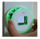
In the event Setra Lite needs to be removed for service, first remove the front lens. To remove the front lends, grab the front lens from the left and right side edges, and pull the lens away from the wall.
