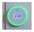
If pressure exceeds alarm limit thresholds, the LED light ring will glow red and an audible alarm will sound for units equipped with audible alarm option.
