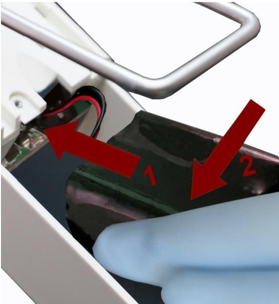
Step 5 – Carefully push battery into the compartment using an upward motion until bottom of battery clears edge of the compartment and drops in freely.
