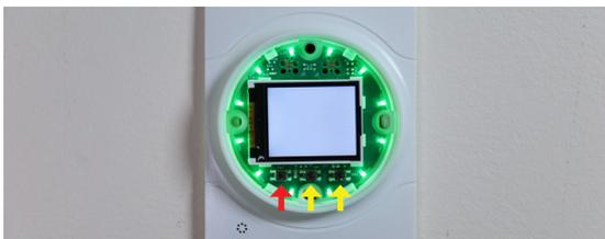
Press and hold the LEFT button for 3 seconds to access the configuration menu (the LED ring should shut off after the configuration menus are accessed).
