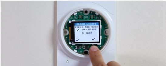
Press and hold the RIGHT button ("✓") to adjust the alarm limits (i.e. pressure at which the LED ring will turn red); the screen text will flash 3 times to indicate that the setting is ready to be adjusted.
