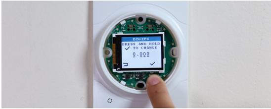
Press and hold the RIGHT button ("✓") to adjust the number of decimal places displayed on the LCD screen; the screen text will flash 3 times to indicate that the setting is ready to be adjusted.
