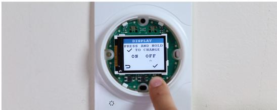
Press and hold the RIGHT button ("✓") to adjust display behavior (i.e. whether the LCD display shows the digital pressure reading by default); the screen text will flash 3 times to indicate that the setting is ready to be adjusted.
