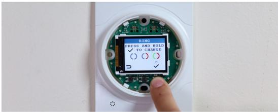
Press and hold the RIGHT button ("✓") to select between no ring light, alarm (red) ring light only or both green/red light ring indicators. The screen text will flash 3 times to indicate that the setting is ready to be adjusted.
