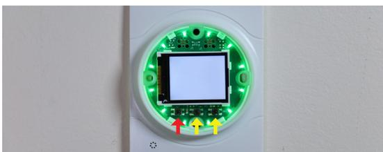
Press and hold the LEFT button for 3 seconds to access the configuration menu (the LED ring should shut off after the configuration menus are accessed).
