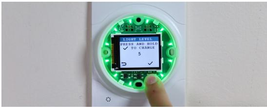
Press and hold the RIGHT button ("✓") to adjust the brightness of the LED light ring; the screen text will flash 3 times to indicate that the setting is ready to be adjusted.
