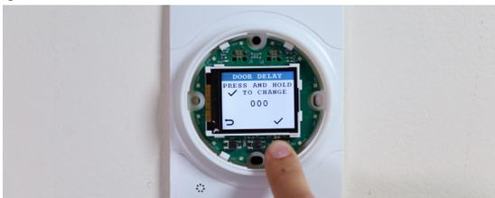
Press and hold the RIGHT button ("✓") to adjust the alarm door delay (i.e. number of seconds before the LED ring will turn red when pressure alarm limits are exceed); the screen text will flash 3 times to indicate that the setting is ready to be adjusted.
