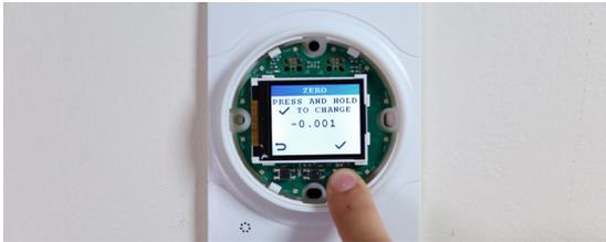
Press and hold the RIGHT button ("✓") to zero the onboard pressure sensor. The unit contains an onboard valve to automatically equalize the pressure differential across the sensor.
