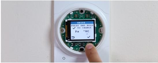
Press and hold the RIGHT button ("✓") to adjust the measuring units used for the digital display and alarm thresholds; the screen text will flash 3 times to indicate that the setting is ready to be adjusted.
