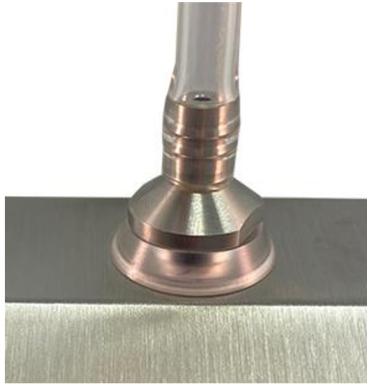
Figure 3-5 Attach Optional Isokinetic Inlet to Joint Tube
