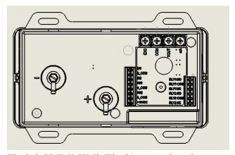
Fig 3-2 SRIM2 Wall (Flush) mount housing rear view of pressure fittings and electrical terminations
