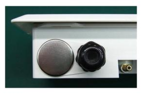
Fig. 3-8 Installed plugs on unused openings in the base.
