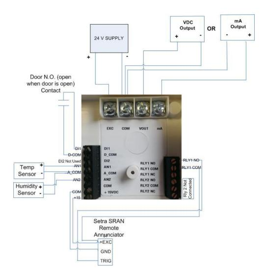
Figure 3-7 Wiring, SRIM2
