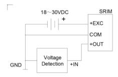
Fig. 3-5 Wiring Diagram SRIM1 and Back of unit
