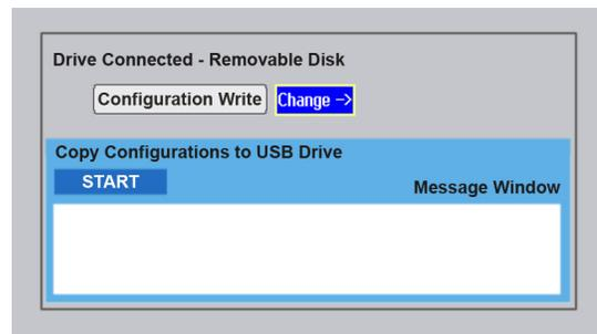
Remove the thumb drive and cable and move to the first “slave” unit to be configured. With power applied to that unit, connect the thumb drive and cable. Select Configuration Read and START to write the master configuration to the new slave unit.
