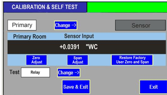
1. Select Primary or Secondary room. When selected, the gray box to the right will indicate if the calibration will be applied to the on-board sensor or the external sensor (Analog Ch1 or Analog Ch2). The indicated pressure is shown.
