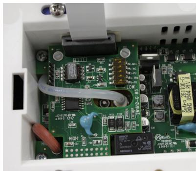
5. After calibration, replace the red and clear tubing.
