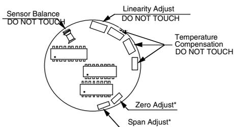
NOTE: When circuit cover is removed, a zero shift can be noticed. The zero will return by the same amount when the cover is replaced. This displacement of the output should be taken into account when making adjustments or during recalibration.
