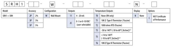
Ordering Example: SRH12PW11TONC = Model SRH, 2% Accuracy, Wall Mount, 4 to 20 mA Output, RH only, No Display, NIST Certificate of Conformance
