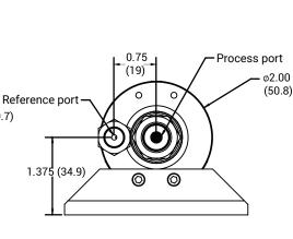
Fitting code "FF" with bayonet connector "B3"
