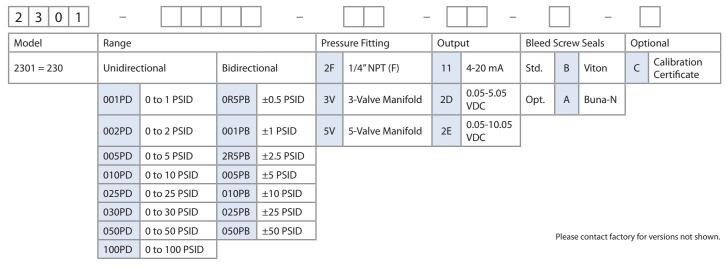
Ordering Example: 2301005PD2F11B = Model 230 0 to 5 PSID unidirectional, 1/4-18 NPT Ext. fitting, 4 to 20 mA Output, and Viton/Silicone Seals. 2301005PD3V11B = Model 230, 0 to 5 PSID unidirectional, 3-Valve Manifold, 4 to 20 mA, Output, and Viton/Silicone Seals (Assembled w/3- Valve Manifold).
