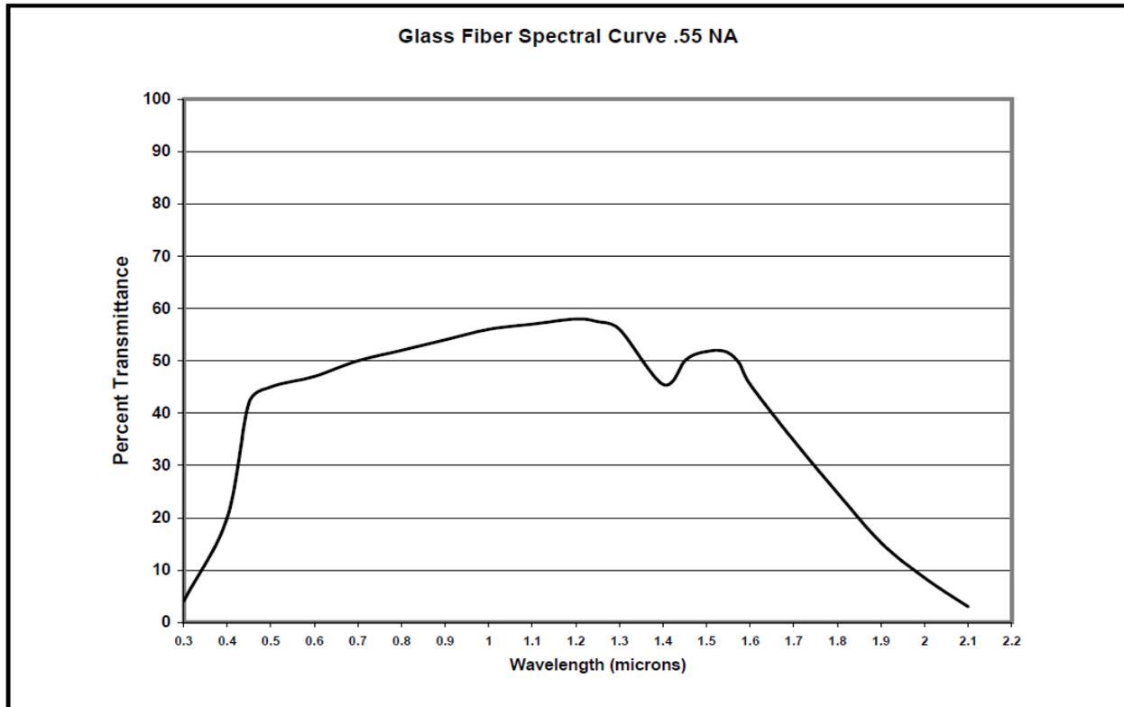
Spectrum shown is for the fiber optic only, and is not representative of output spectrum when paired with a light source and lensing.
