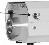
4. With the screws loosened, rotate the top cover locks downward in the slots in the cover.
