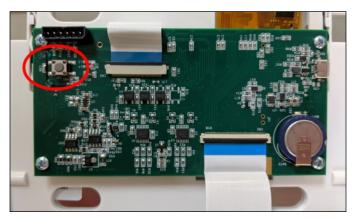
Caution: Resetting a unit to factory default, either via the configuration menu or via the physical reset button, will result in all configuration settings being erase.
