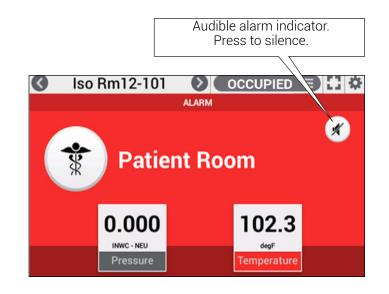
**Audible Alarm** Enabled causes an alarm condition to sound the audible alarm behind the FLEX faceplate. When Disabled, FLEX will still annunciate the alarm via a relay, visibly on the FLEX screen, and over the network to a BACnet object. The relay is configurable, and may not always annunciate when in alarm. The audible alarm volume is 68 dBA.
