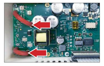
Adjust Span is used for calibration of the internal or external pressure transducer sensor and testing operation of hardware circuitry. Calibration using Adjust Span is only required for highly accurate measurement needs such as those needed to comply with federally mandated regulations. Calibration should only be performed by qualified personnel, using a pressure calibrator such as the Setra MicroCal or equivalent.
