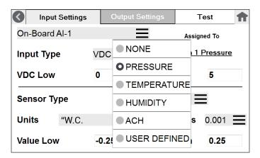
When the Sensor Type is chosen, the input signal can then be scaled using Low and High signal values that match the full-scale range of the applicable sensor. In the example below, these are "mA Low" and "mA High." This scaling of the input allows the sensor's output signal to be scaled to the desired reading on the Home screen. Select the Engineering Units "Eng Units" and define the full-scale range of the sensor in the appropriate units of measure.
