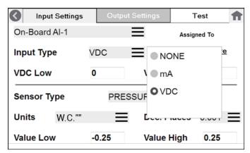
Choose the Sensor Type being used. Pre-selections are available for Pressure, Temperature, Humidity, and Air Changes per Hour (ACH). A User Defined selection can also be chosen if the sensor is not one of the ones on the pre-selected list.
