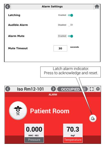
**Latching** is an alarm function that causes an alarm condition to persist even when the Badge parameters have returned to normal operating ranges. A Latched alarm must be acknowledged at the FLEX touch screen interface itself to be cleared. This function is useful when it is important for staff to be physically present at the room to observe the alarm condition and respond to it.
