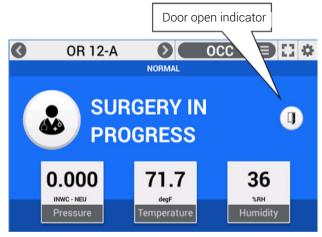
Any of the User Defined badges can also display the status of the DI. To configure the User Defined badge as a DI, select Digital as the Input Type on the User Defined badge set up screen. Enter the desired text for the Inactive and Active status of the DI which will be shown on the Badge.
