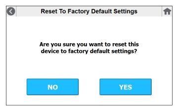
An alternative way to reset the unit to factory default settings to press and hold the physical reset button on the display circuit board for 150 seconds. For units where a Supervisor Passcode is set and forgotten, this is the only method to recover access to the configuration settings on the unit.
