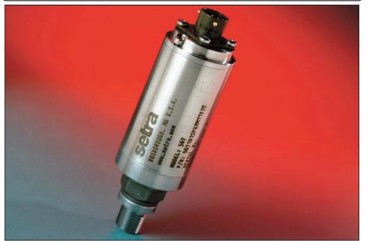
S etra's Model 567 high performance pressure transducer offers customer accessible down-ranging capabilities, making this unit ideal for high overpressure applications. The 5:1 turndown is easily accessed via a switch and potentiometer.
